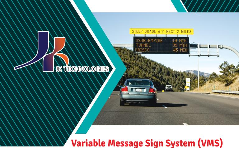
Variable Message Signs (VMS) are digital road signs used to inform car drivers about specific temporary events and real-time traffic conditions. The signs are often linked to a manned control centre via a local network. Variable message signs (VMS) are a vital part of Intelligent Transportation Systems.
